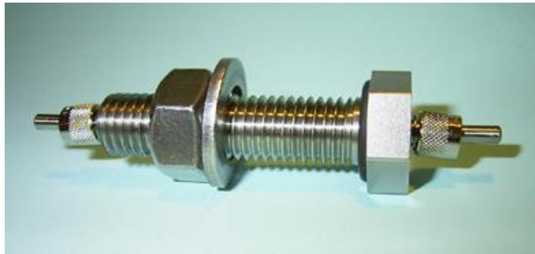
The FC-VFT vacuum feedthroughs are designed for use of fiber optics in vacuum chambers, such as for plasma monitoring. The vacuum feedthrough consists of an M12 housing with Viton® O-ring and 2 SMA fiber optic interconnects to allow easily coupling to fiber optic cables and probes. The vacuum feedthrough can be delivered for all fiber diameters, such as 50 μm up to 1000 μm for UV/VIS as well as for VIS/NIR. (This is a product of Avantes, Inc., Boulder, Colorado.)
